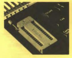
Now Watford Electronics brings you a ROM board for small budgets or for those of you who do not wish to open up your Micro frequently. It allows you to change ROMs quickly and efficiently with the minimum of effort – no screws to loosen or keyboard to remove. The unit consists mainly of a zero insertion force (ZIF) socket on a small circuit board which is located into the position of the 'ROM Cartridge' and is connected to one of the internal ROM sockets via a ribbon cable.
